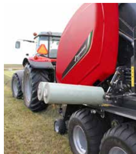
Twin satellite wrapper with two pre-stretchers and four endless belts for fast and reliable wrapping.
