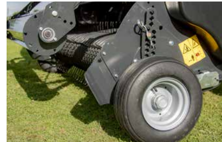
Generous flotation tyres with easy height adjustment.
