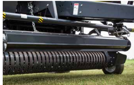
Large diameter roller crop press facilitates crop flow at high intake speeds.
