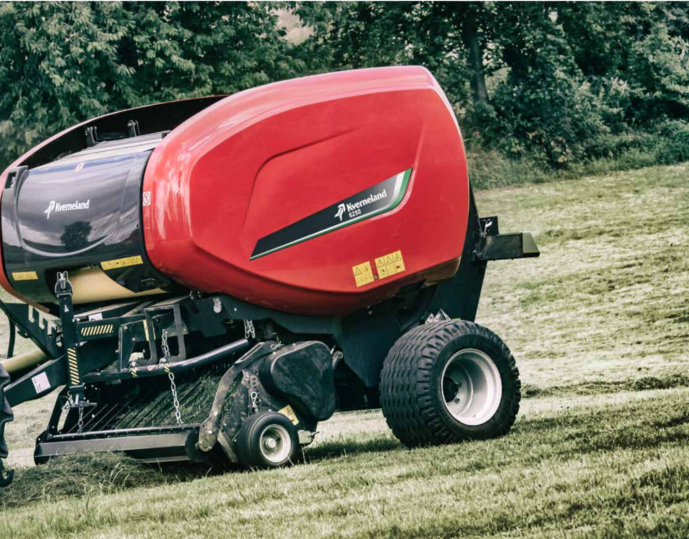
Drop Floor in working position.
