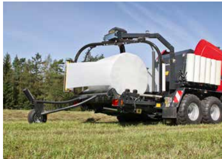
Twin satellite wrapper with two pre-stretchers and four endless belts for fast and reliable wrapping.
