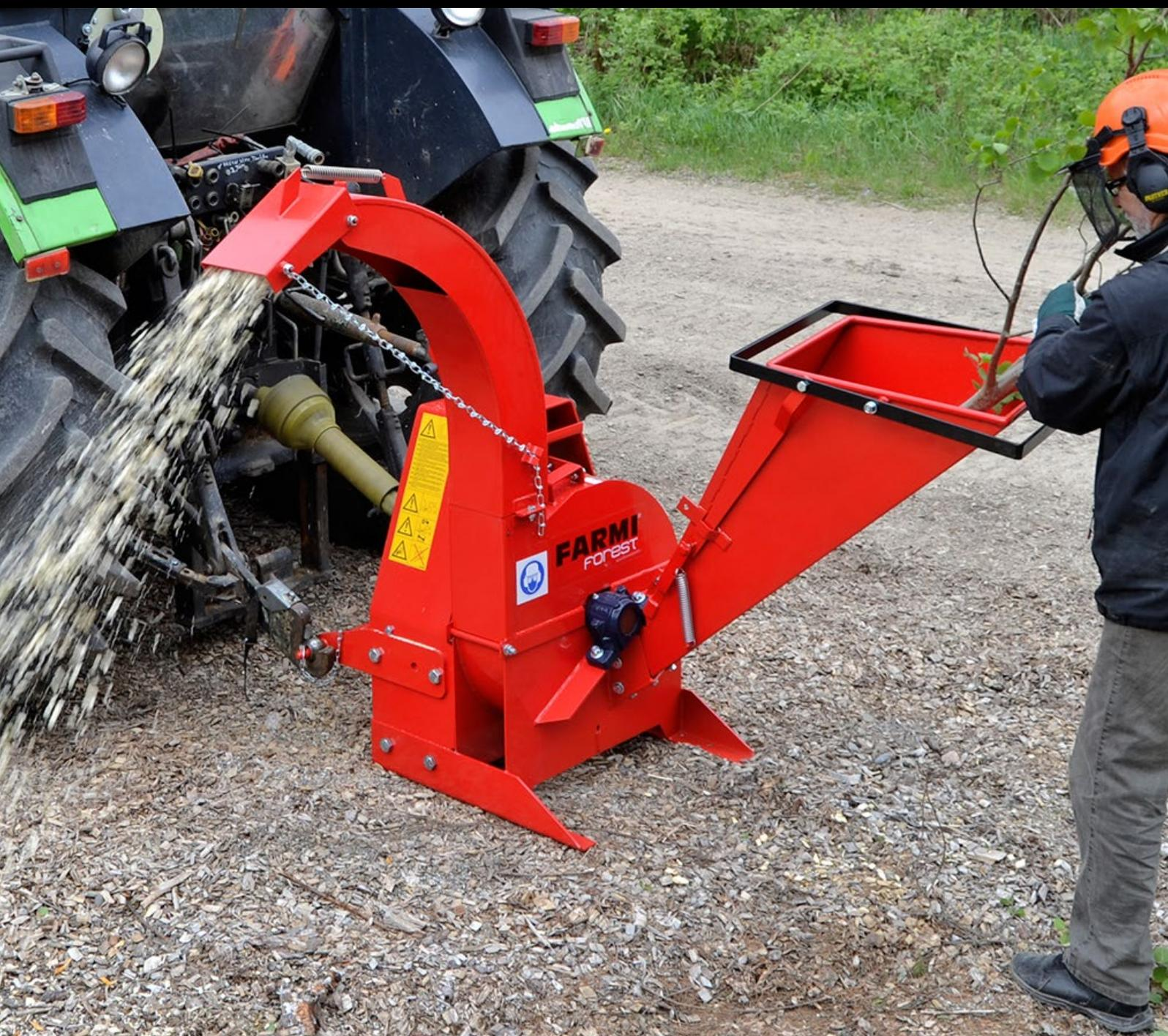
**FARMI CH 100 F** is designed as a robust and inexpensive disc chipper for landscaping to chip branches and small trees up to a diameter of 100 mm. The FARMI CH 100 F can be mounted onto a small tractor giving a compact chipping machine in gardens, parks, yards and road sides. Two knives and an anvil take care of chipping and feeding. CH 100 F chipper is available as a tractor PTO versions or as a hydraulic driven option.
